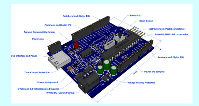
Currently restricted to two PICs: The PIC18F25K20 (3V) and the PIC18F25K22 (5V) These are 32K flash devices operating at 64MHz.
