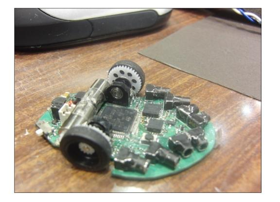
Four Wheels, stepper motors, half size. How hard does it need to be?
